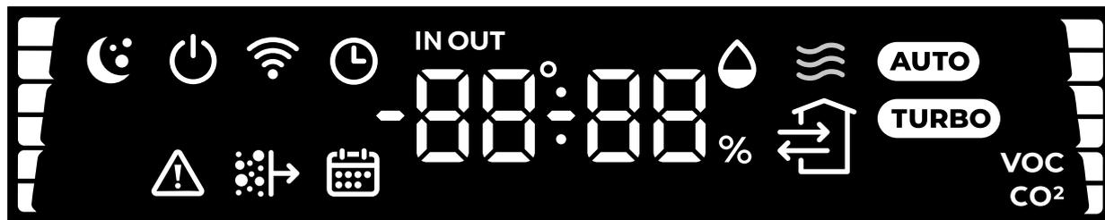
The digital segment of the display shows information such as time, temperature, humidity or all of them in sequence. You can also select the temperature sensor to display (outdoor, supply air, indoor) and select a CO<sub>2</sub> or VOC sensor. The scale on the right shows the fan speed. The scale on the left shows the air quality.
