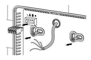
**5.** Remove the connector with the cable from the bracket and connect it to the female connector on the circuit board.
