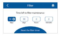
Setting the filter maintenance timer: upon elapsing of a pre-set period of time (70–365 days) the main page will show a filter replacement alert while the **Alarms** window will display the respective information about the necessary filter change. To disable the filter timer (e.g. if the unit is equipped with pressure switches), set the value to 0 days.
