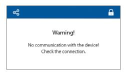
If the RS-485 network parameters are set incorrectly or if there is a problem with the cable, the display will show a warning ("No communication with the device. Check the connection").
